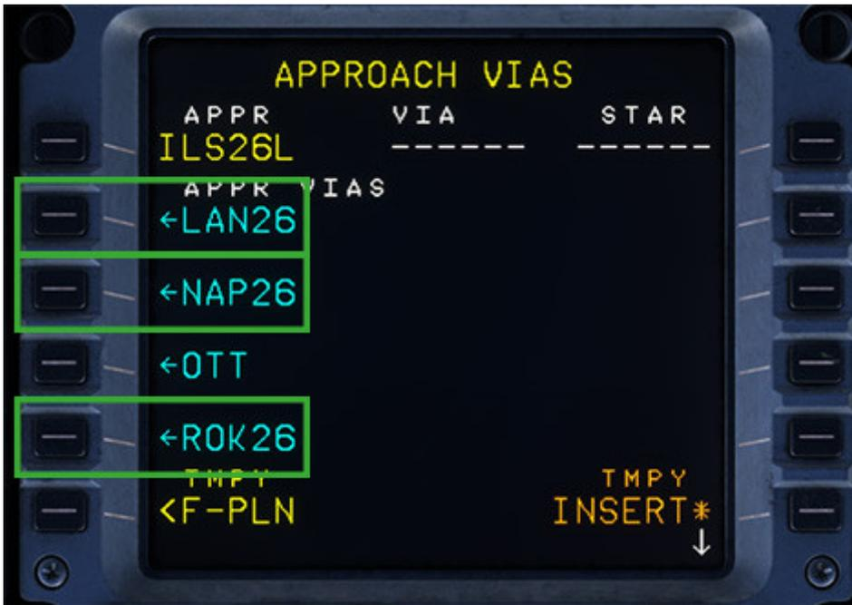
Finally, check that your FMC is correctly displaying the up- and downwind as per the published charts. If things are programmed correctly, you will not have MIQ or OTT in your flight plan. **If you are unsure, or things look weird, inform your controller!**
