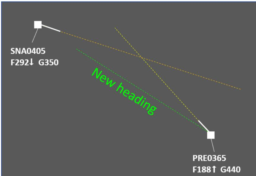
An example of using vectoring and vertical speed control. Turning PRE0365 provides safety and assigning vertical speeds results in efficiency as the flight can be returned onto the flight planned route sooner.
