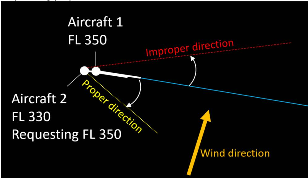
Turning Aircraft 2 to the right allows it to safely climb to FL 350. Due to the speed reduction caused by the wind Aircraft 2 can be sequenced behind Aircraft 1.
