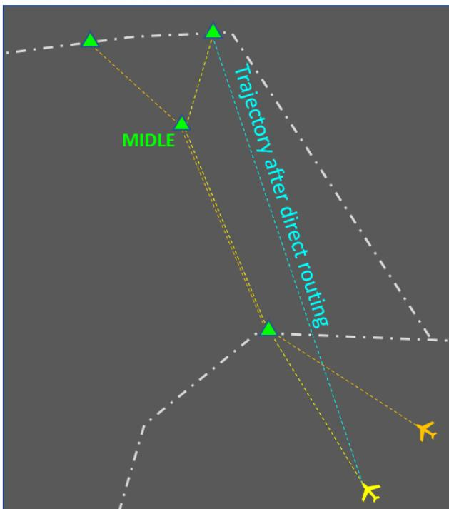
An example of using a direct route and a level change. Initially, the conflict is of the converging type. By clearing the yellow aircraft to fly on a direct route, the controller does not solve the conflict but now has the option to use 1000 ft level change for a few minutes as opposed to 2000 ft until point MIDDLE.
