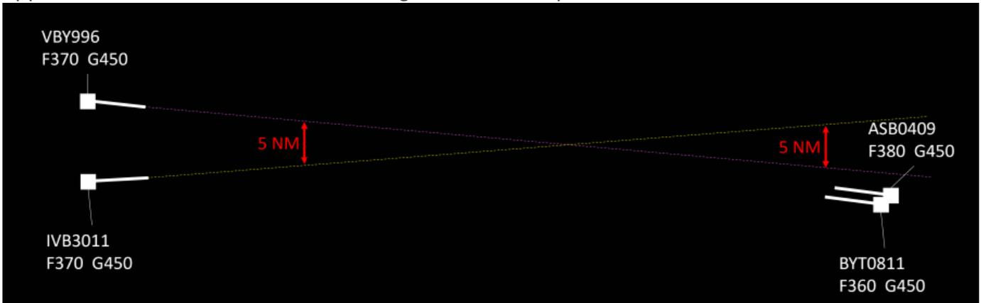
The use of opposite levels can sometimes be justified when the conflict is at the sector exit point. This solution, however, is subject to approval from the downstream controller. The feasibility of this option depends on the geometry of the conflict (are the aircraft diverging after the point of conflict) and on the traffic situation (are there aircraft that are flying at the same level on an opposite track).
