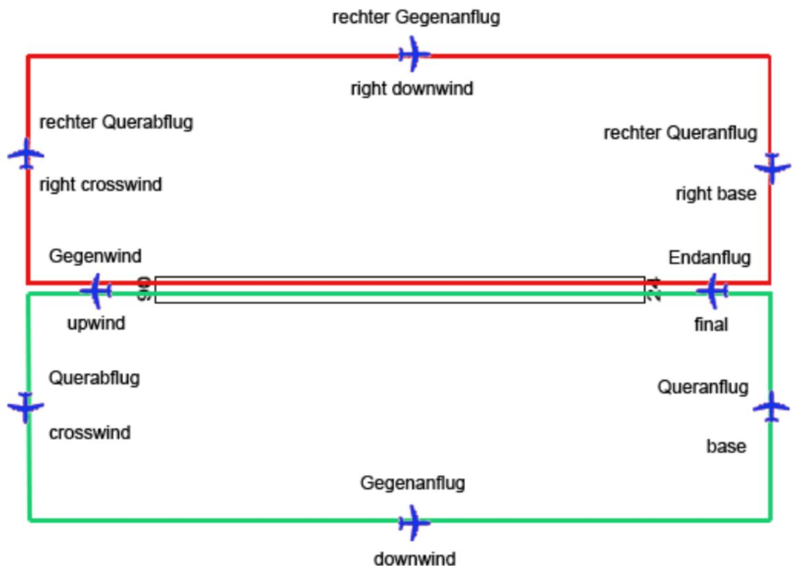
If we mention "traffic circuit", a "crosswind", "downwind" or "base", this refers to the sections of the **standard traffic circuit** (left turns).
